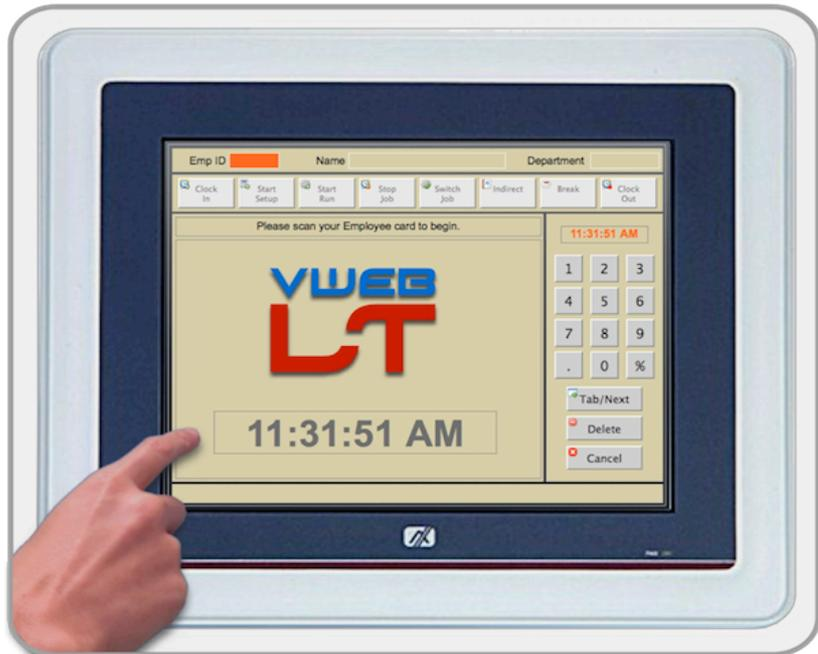
VWEB-LT is a real-time shop floor data collection solution for labour tracking and provides both paperless and paper-based shop floor control.
